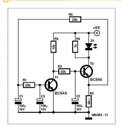
Operation is largely independent of supply voltage, and the average LED current is set at about 10 mA. The circuit adjusts the voltage across the emitter resistor so that it matches the base voltage of the first transistor (around 0.6 V). The phase shifting network gives rise to the oscillation around this average value.
